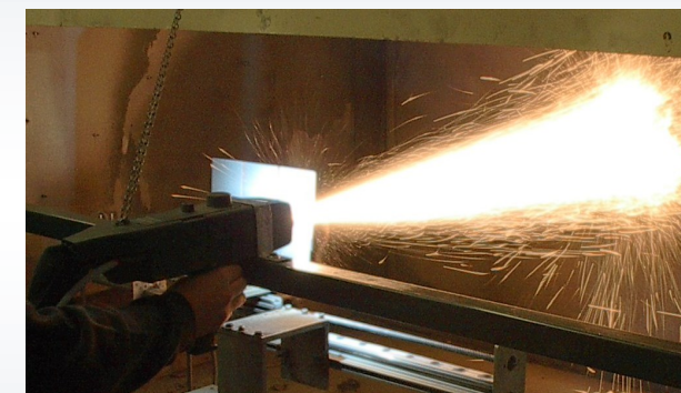
Twin Wire Electric Arc spray process
