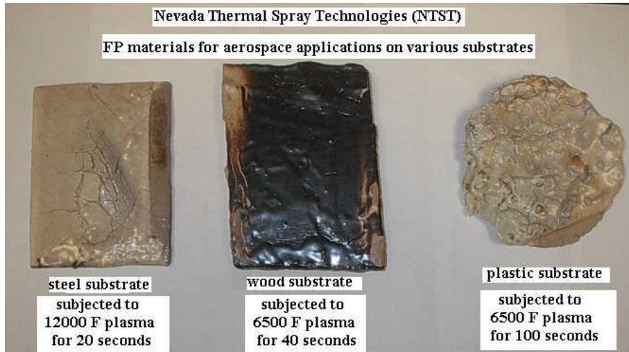
Figure 3. High Temperature Testing of NTST TP Coatings.
